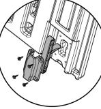
Latch-1 (GS0201018)x1pcs Latch-2 (GS0201019)x1pcs Crosshead screw Q2540410 M4x10x4pcs
