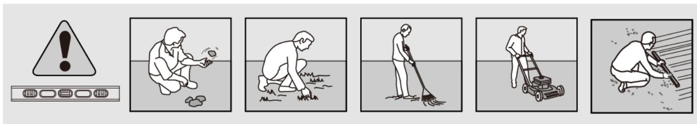
Level the ground surface before unpacking parts and beginning assembly.
